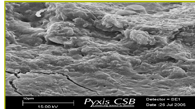
Cracks and fissures on surface of oxidised, hydrophilic film
